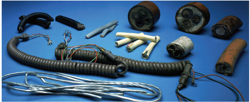
FIGURE 1. Many types of insulated wires can be treated with cryogenic liberation using liquid nitrogen. Other materials that can be cryogenically treated include circuit boards, metal/rubber weather stripping, plated plastics and composite parts.
